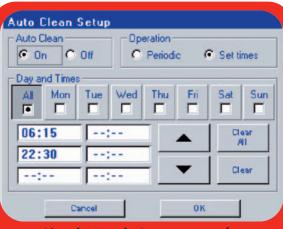
Simple Touch Screen set-up for Automatic Cleaning System.
